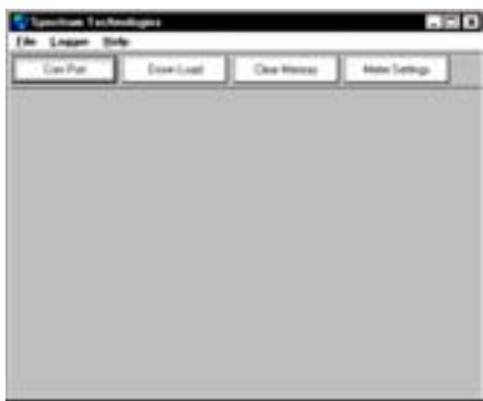
connected to the probe. Use the **Com Port** button to select the port connected to the computer data port. The **Download** and **Clear Memory** buttons are not used with the TDR 100.
